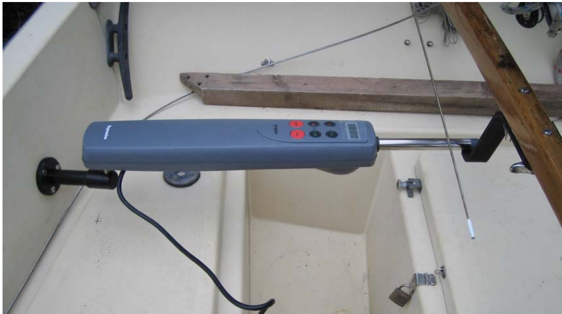
Photo E: New Tiller Pilot in Place
