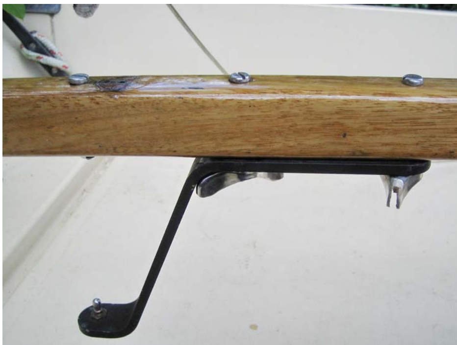
Photo C: Tiller Bracket in New Position
